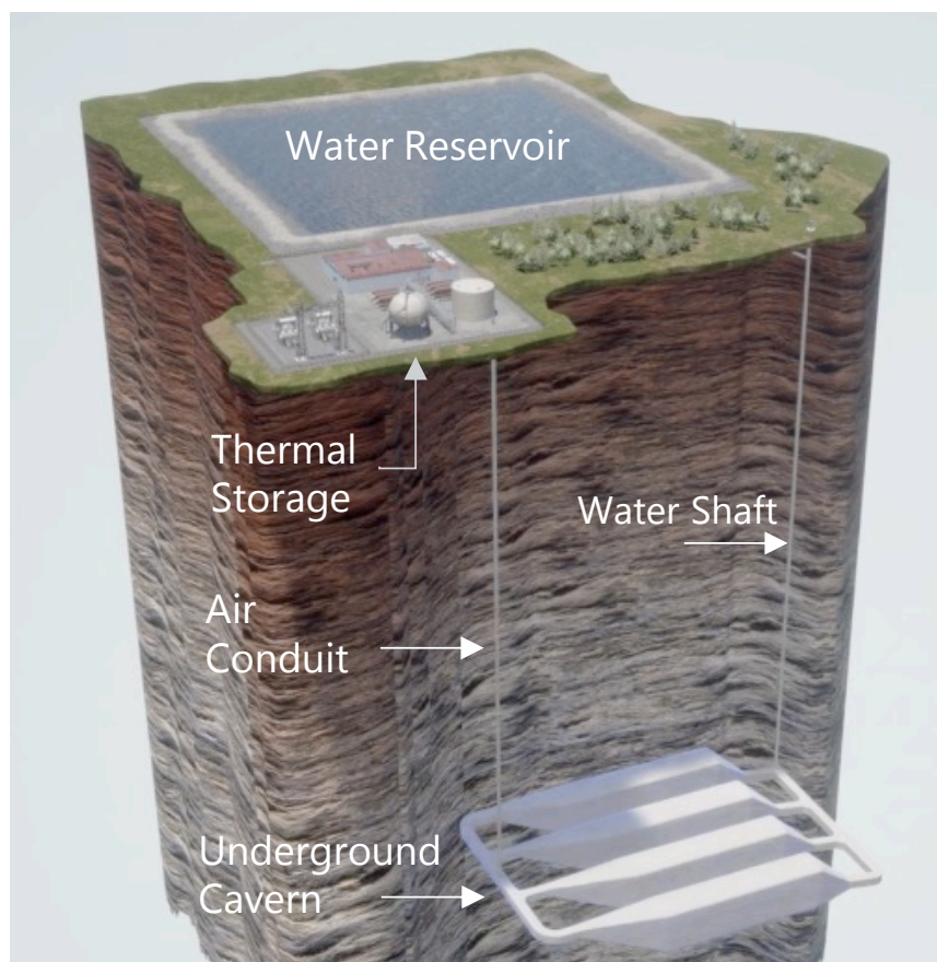
Fig. 2. 7 Schematic of Hydrostor’s advanced compressed air storage approach
