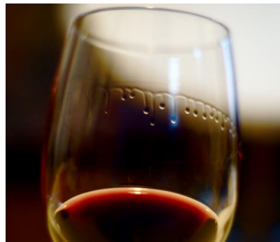
Fig. 25. Illustration of the phenomenon of tears of wine along the wall of a glass containing ordinary table wine.
