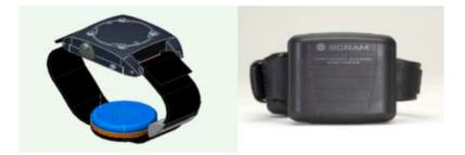
Figure 1: Alcohol Biosensor Devices: The WrisTAS (left) and the SCRAM (right).
