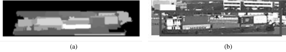
Fig. 9. Saliency detection result of a bounding box. (a) The salient region. (b) The location of the ship.
