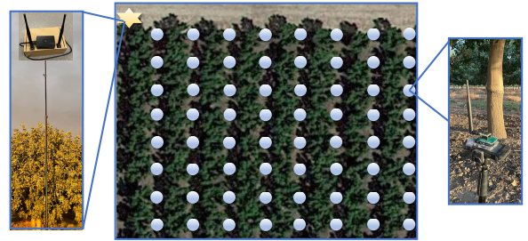
(b) The setup in one area (one gateway and M locations).
